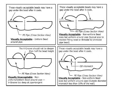
Figure 3 – Outside Diameter Butt Fusion Bead Guideline as per ASTM F2620
