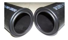
Figure 2 - Unacceptable Concave Melt Appearance
