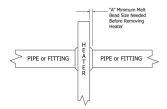
Table 1 – Melt Bead Sizes for Corresponding Pipe Sizes
