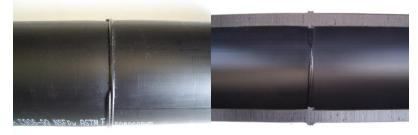
Figure 8 - Incomplete facing or insufficient heat time
