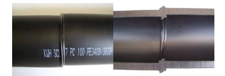
**Figure 7** - Pipe misalignment (high-low misalignment)
